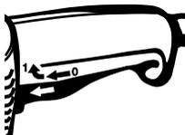
TO SWITCH TOOL "OFF": Release pressure on paddle lever. The switch is spring loaded and will return to "OFF" position automatically.
